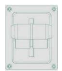
T-bar is for performing effect transitions manually. It can be either all the way up, all the way down, or anywhere in between. To enable SE-800 T-Bar, the T-Bar on RMC-90 need to be set at either end of its travel.
